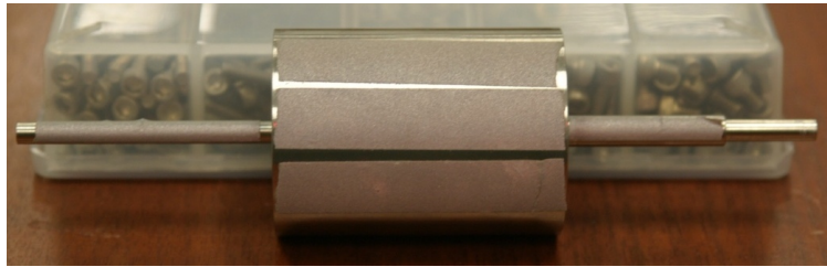
Figure 68. Rotor with Reflective Tape for Ping Test
