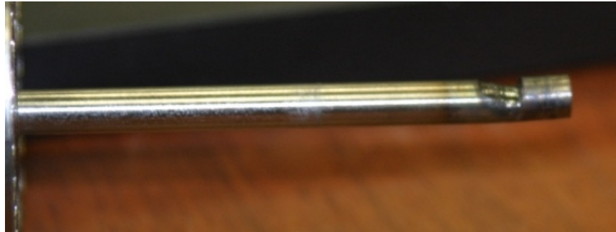
Figure 78. Rotor Shaft After Spin Up, Zoomed
