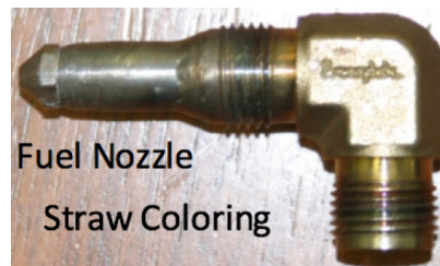
Figure 65. Fuel Injector with Straw Coloring After Burner Testing
