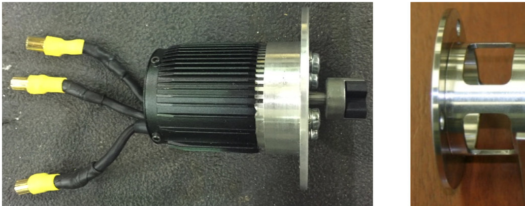
Figure 23. Upper Half of the Motor Mount (left), Lower Half of the Motor Mount (right)
