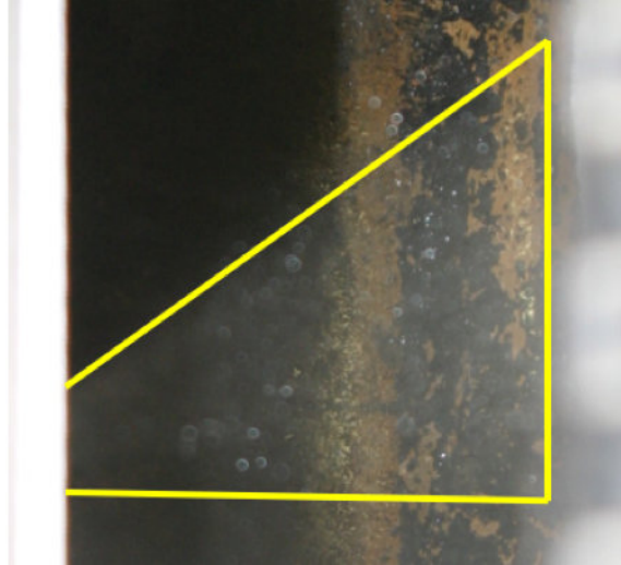
Figure 37. Devalan Nozzle Spray Cone Half-Angle Highlighted
