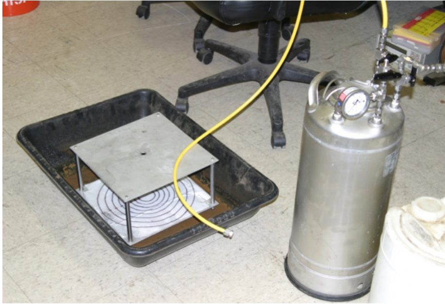
Figure 36. Test Set-up of Peanut Injectors
